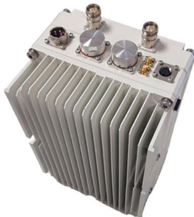
Figure 54: Illustration of the 5G RAN gNB Remote Radio Unit (RRU) unit.
