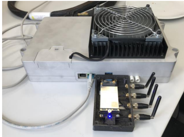
Figure 62: 5G connectivity to the tractor controller.
